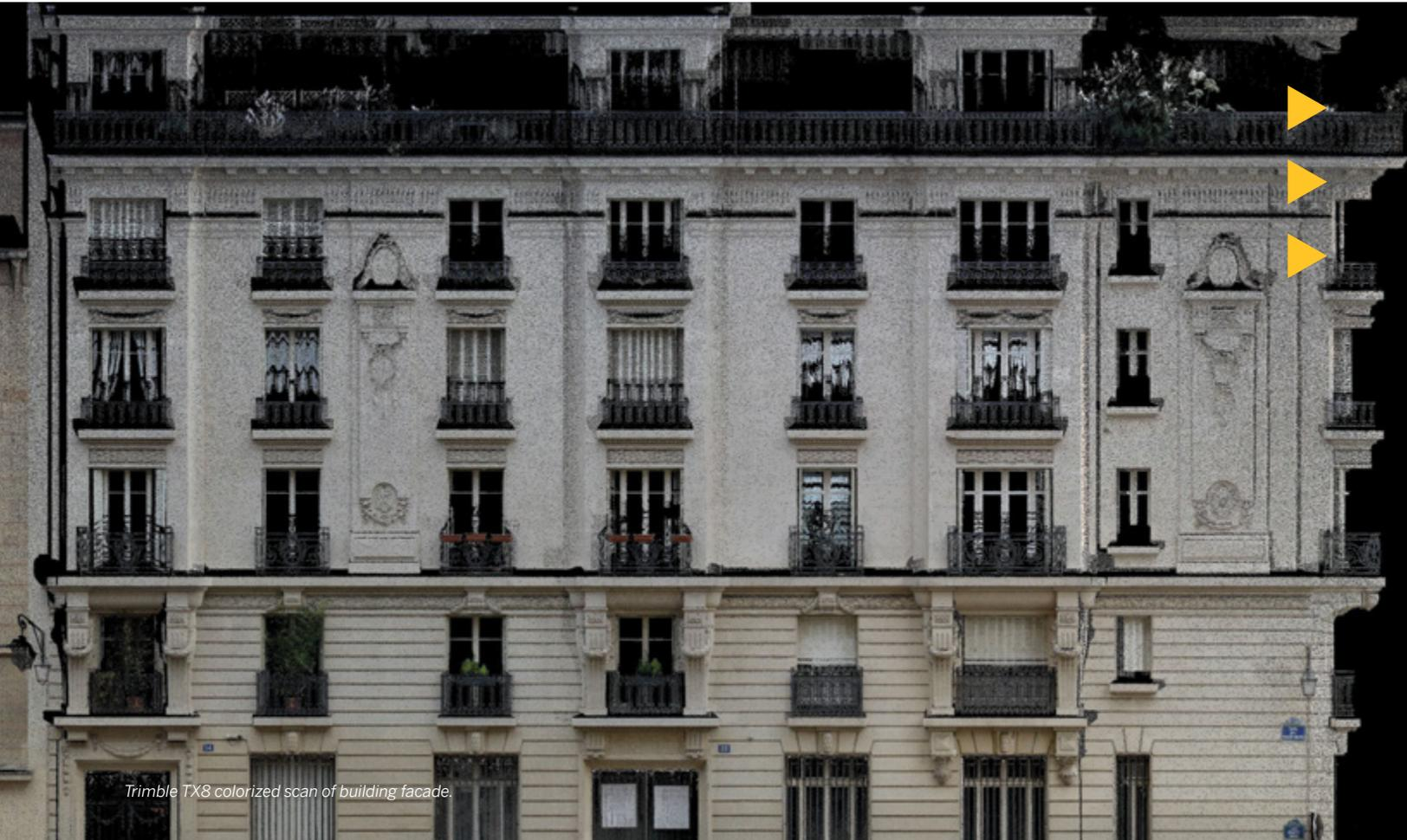
Trimble TX8 colorized scan of building facade.
