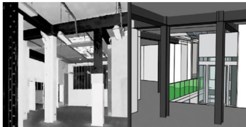
*Trimble TX8 scan of original entrance and SketchUp model of new elevator to the basement.*
