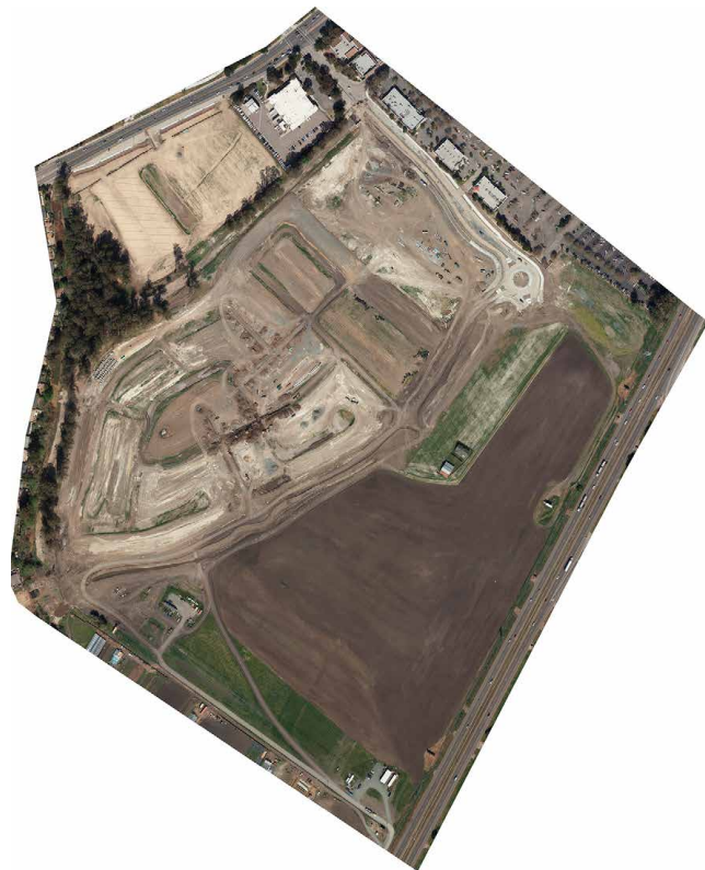
Above: The finished orthophoto mosaic from 2020. CCAM used Inpho OrthoVista to automatically stitch together the 23 orthorectified images.
